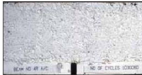
Reinforced sample and still no significant cracking > 1,000,000 load cycles
